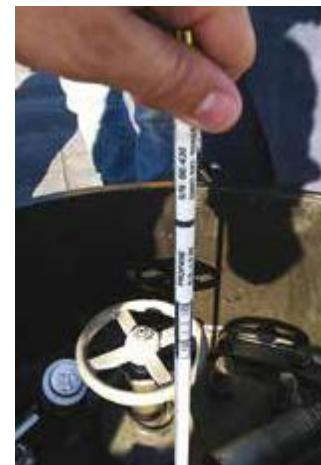
**STEP 10:** Convert the gauging device reading to gallons, using the outage table for the tank car. Subtract the outage in gallons from the water capacity of the tank car and record the result on the company unloading form.
