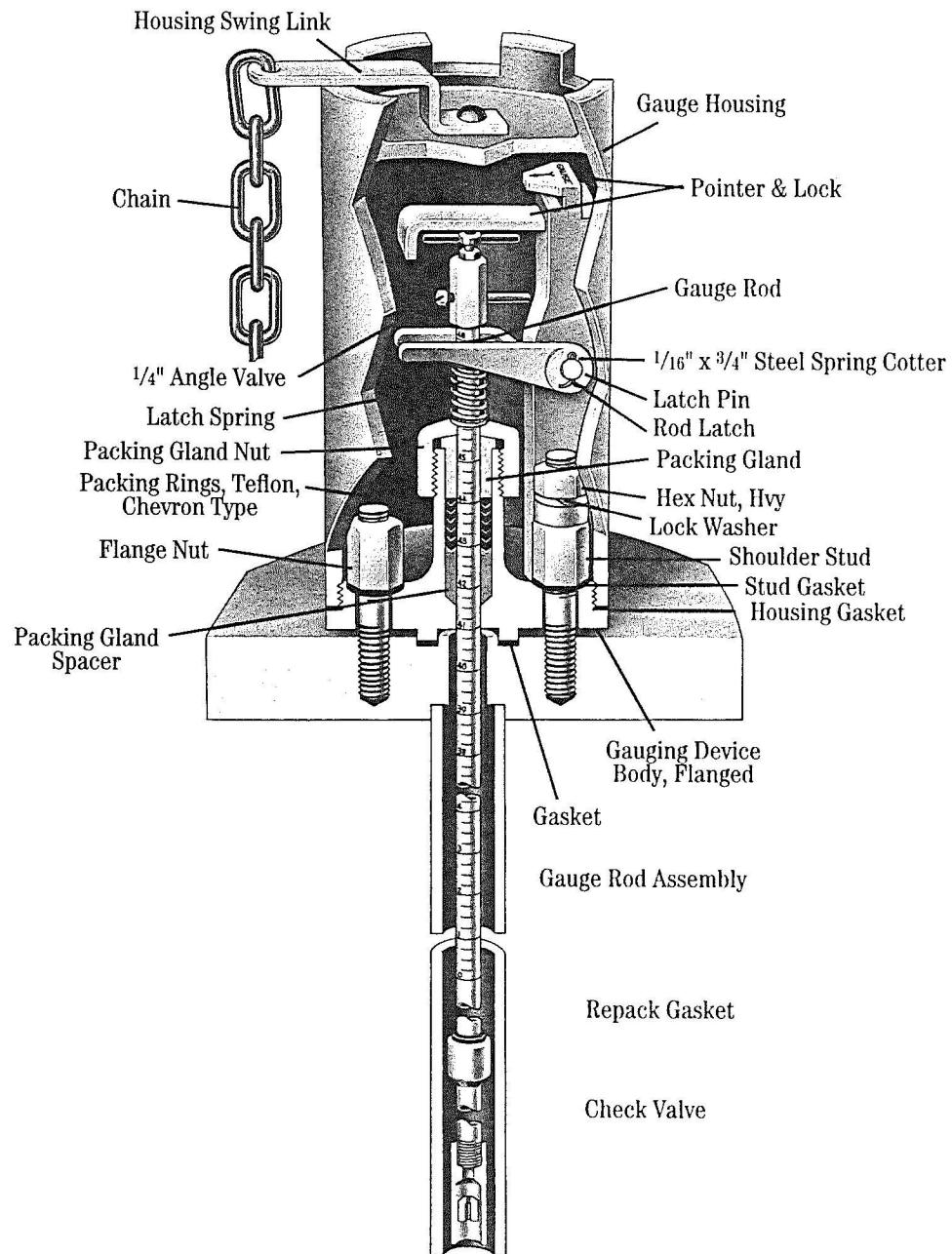
**"SLIP-TUBE" GAUGING DEVICE ASSEMBLY
