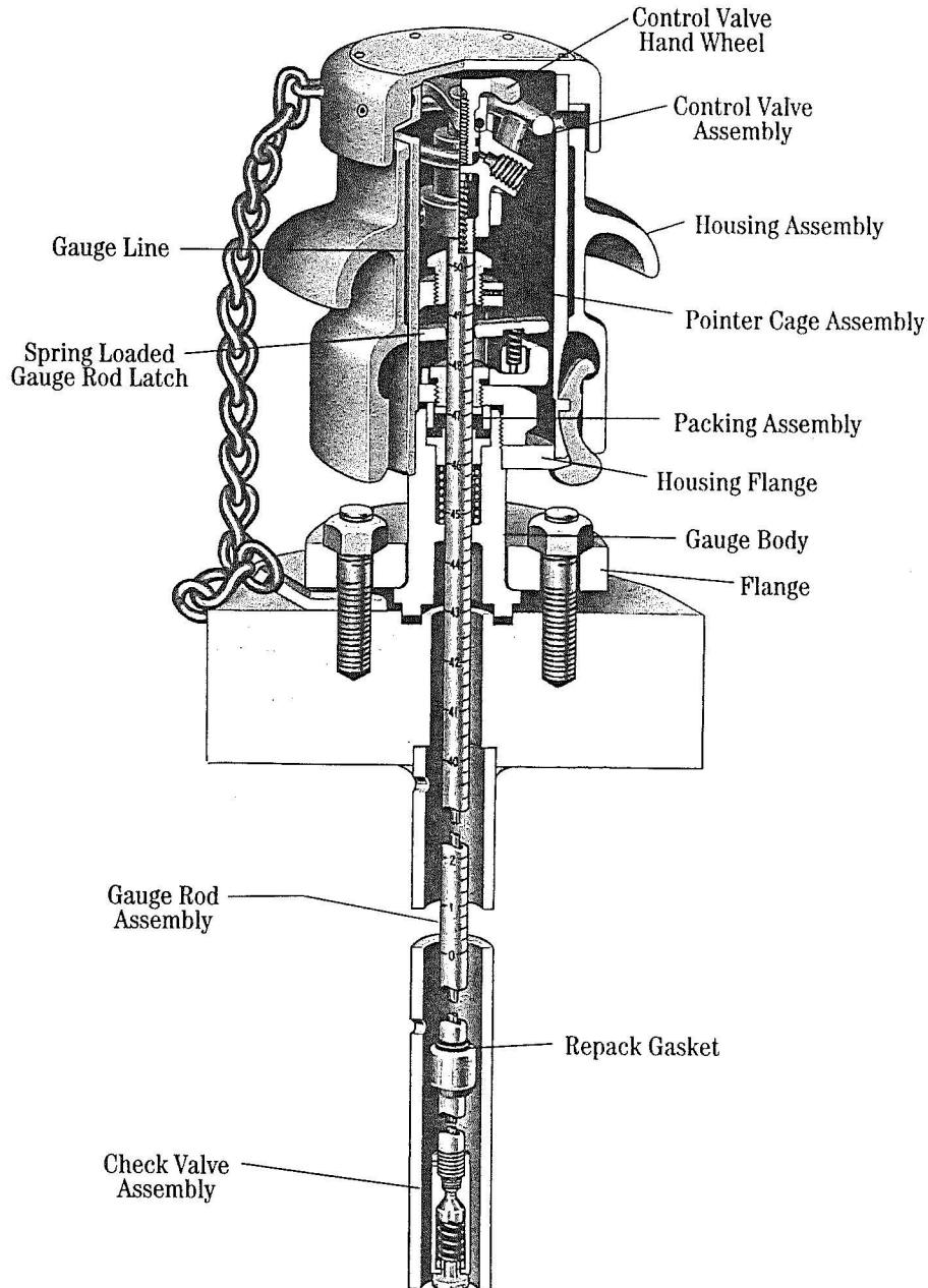
**"SLIP-TUBE" GAUGING DEVICE ASSEMBLY
